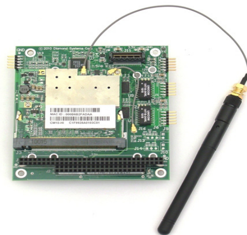
Corona SUMIT Communications module with external antenna installed
